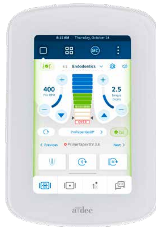
The integrated Midwest apex locator accurately identifies—and shows—the file position relative to the canal apex on the DS5 touchscreen as you work.
