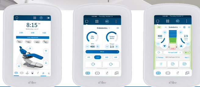
Upgraded DS5 touchscreens show: chair position, RPM and torque, and apex locator (with Midwest)
